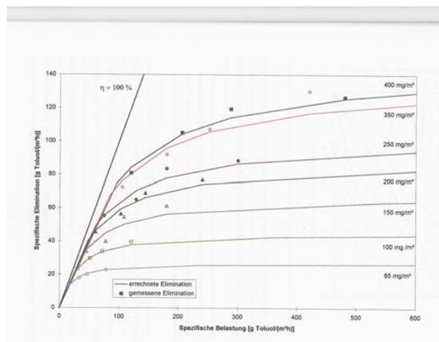
Regarding the data in the given drawing, you can see the difference between calculated data and measured data in pilot tests.
