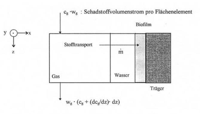
Under steady state conditions the difference between mass flow rate before and after the volume element must be equal to the mass flow rate in the liquid phase and the biological layer.
